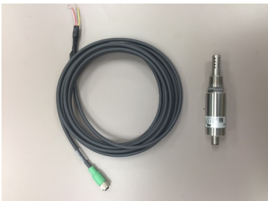
Figure 15 E+E Moisture Probe
